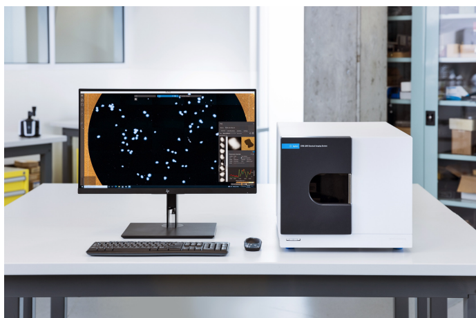
Figure 1. The Agilent 8700 LDIR Chemical Imaging System allows the high-speed routine analysis of microplastics, including the number of particles present in the sample, and their size and chemical composition.
