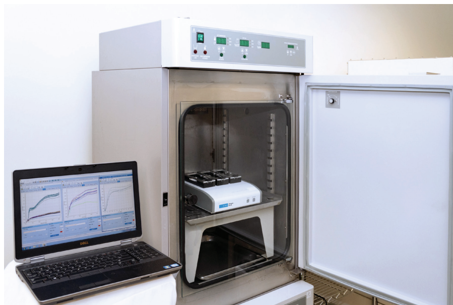
Figure 1. Example of an Agilent xCELLigence instrument. The instrument is placed inside a standard tissue culture incubator, and is compatible with the full range of biologically relevant temperatures, atmospheric compositions, and humidities. The instrument is controlled by a laptop computer stationed outside the incubator.
