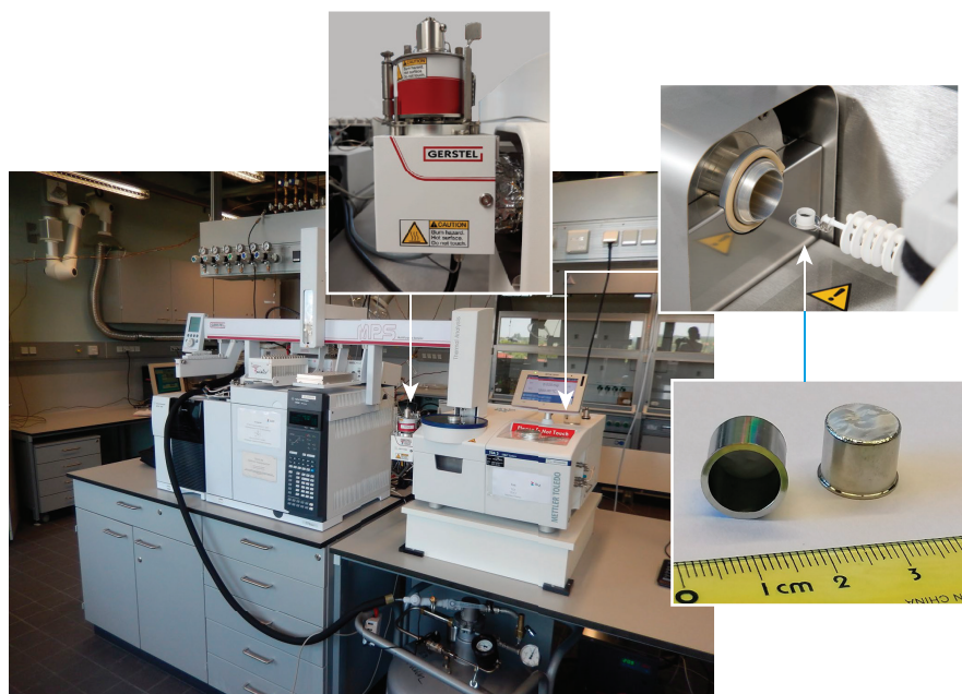
Figure 1. Complete TED-GC/MS instrument setup with the TGA furnace (right) and coupling device (top). The TD-GC/MS system based on the Agilent 5977B GC/MSD (left), and sample robot. The patented smart filter crucible is shown bottom right. Photos courtesy of BAM.
