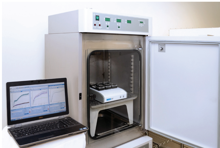
Figure 6. Live cell analysis directly inside an incubator. Placed inside a standard tissue culture incubator or hypoxia chamber, Agilent xCELLigence instruments are compatible with the full range of biologically relevant temperatures, atmospheric compositions, and humidities.
