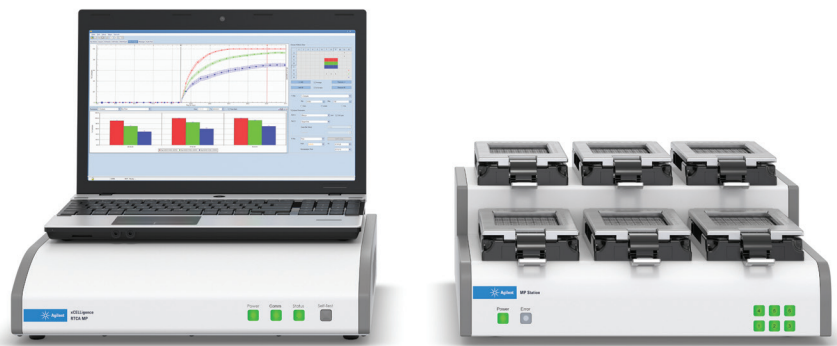
Figure 2. Example of an Agilent xCELLigence instrument. xCELLigence instruments are available in different formats (16-, 48-, 96-, and 576-wells). The instrument shown contains six cradles, each of which houses an electronic 96-well microplate. The plate-housing portion of the instrument is placed inside a standard tissue culture incubator, while the analyzer and control unit (a laptop computer) are housed outside the incubator. All six plates can be monitored simultaneously and independently of one another, maximizing throughput and flexibility.
