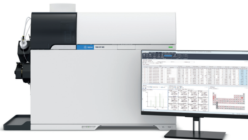
Figure 1. Agilent 7900 ICP-MS with workstation showing latest version of Agilent ICP-MS MassHunter software.
