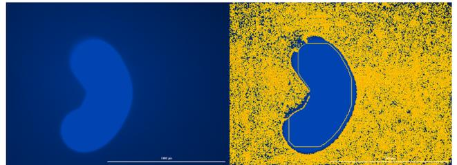
6. Overstaining/overexposure (This example is particularly severe)
