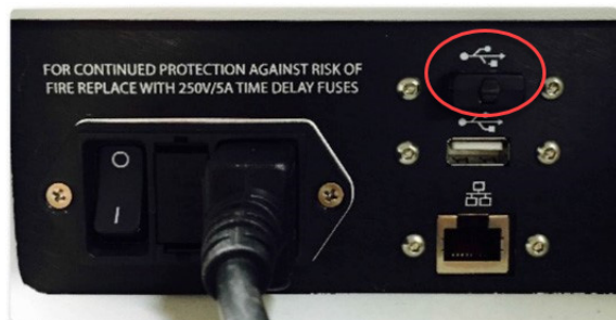
Figure 31. USB WiFi adapter inserted into an available USB port on the back of the XF HS Mini Analyzer
