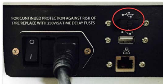
Figure 32. USB WiFi adapter inserted into an available USB port on the back of the XF HS Mini Analyzer
