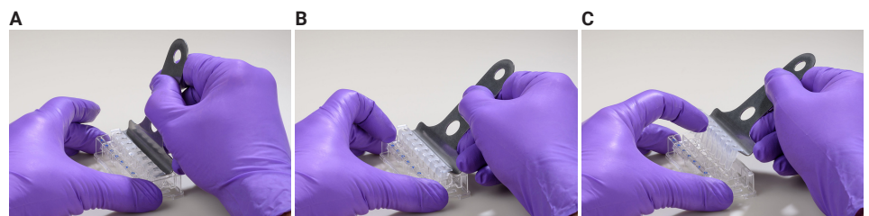
Figure 6. (A) insert the prongs of the removal tool between each well, keeping the bottom of the tool parallel to the top of the plate. (B) once the prongs are inserted, lever the mask from the wells of the plate. (C) Hold the mask onto the removal tool with one finger as it's being lifted from the plate to prevent it from falling.
