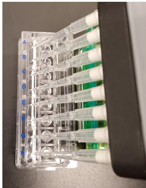
Figure 2. An 8-channel P200 pipettor is used to fill the cartridge moats.
