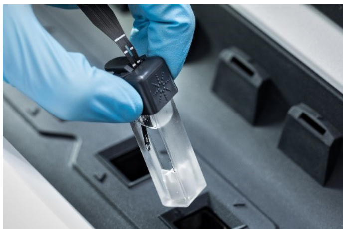
Figure 11. Cary in-cuvette temperature probe has a low mass, large surface area, and a super fast feedback loop.
