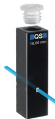
Figure 2. The highly focused beam of the Cary 3500.
