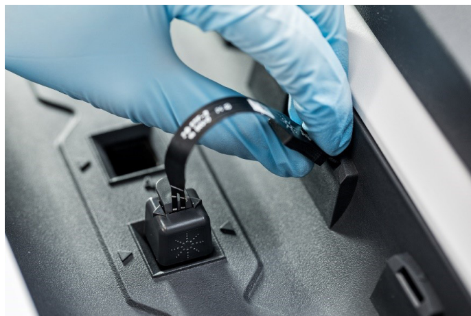
Figure 15. The temperature probe connector plugs into the instrument.
