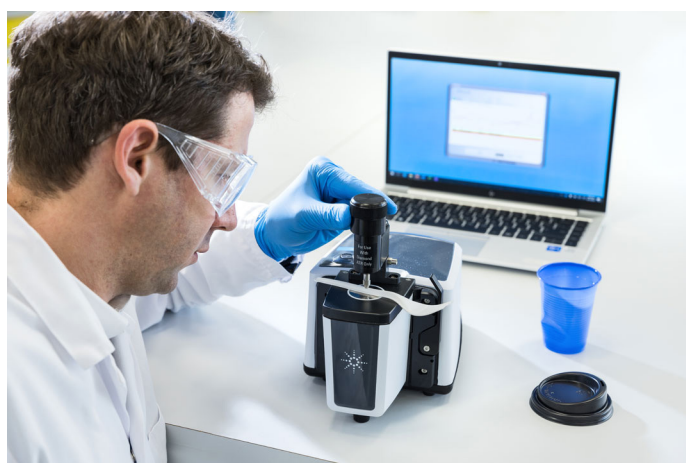
Figure 3. Plastic film and plastic waste analysis using an Agilent Cary 630 FTIR with ATR sampling module.
