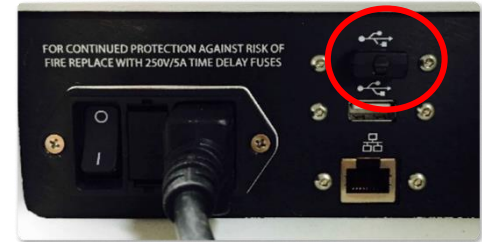
Figure 4 | USB Wi-Fi Adapter inserted into an available USB port on the back of the XFp Analyzer.
