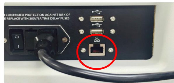
Figure 2 | Ethernet (RJ-45) jack location outlined in red.
