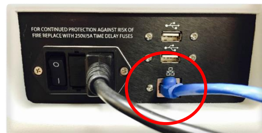
Figure 3 | Wired network connection with Ethernet cable.
