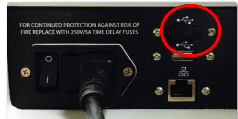
Figure 5: USB Wi-Fi Adapter inserted into an available USB port on the back of the XFp.
