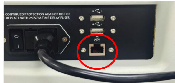
Figure 2: Ethernet (RJ-45) jack location outlined in red.
